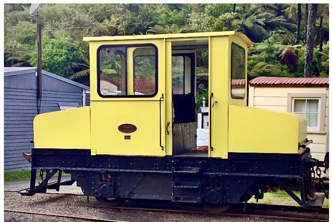
Electric loco used in a factory where steam was no allowed for food production
